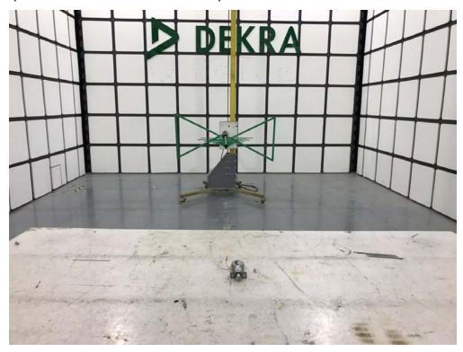
Description: Radiated Emission Test Setup for 1~18GHz
