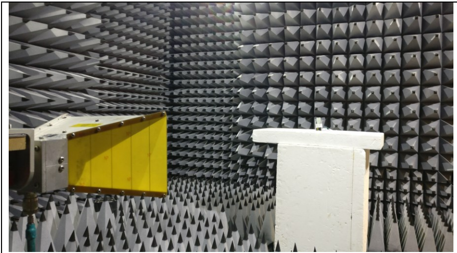
Fig 3 Test setup 1GHz -18GHz Rad Emission
