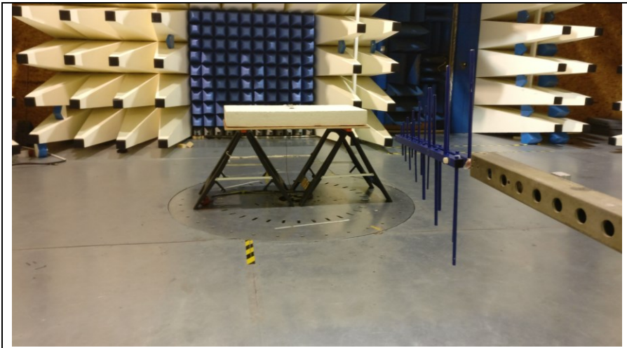
Fig 2a Test setup 300MHz -1GHz Rad Emissions
