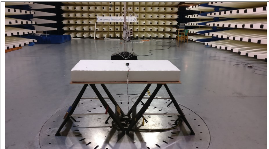
Fig 1b Test setup 30MHz -300MHz Rad Emissions
