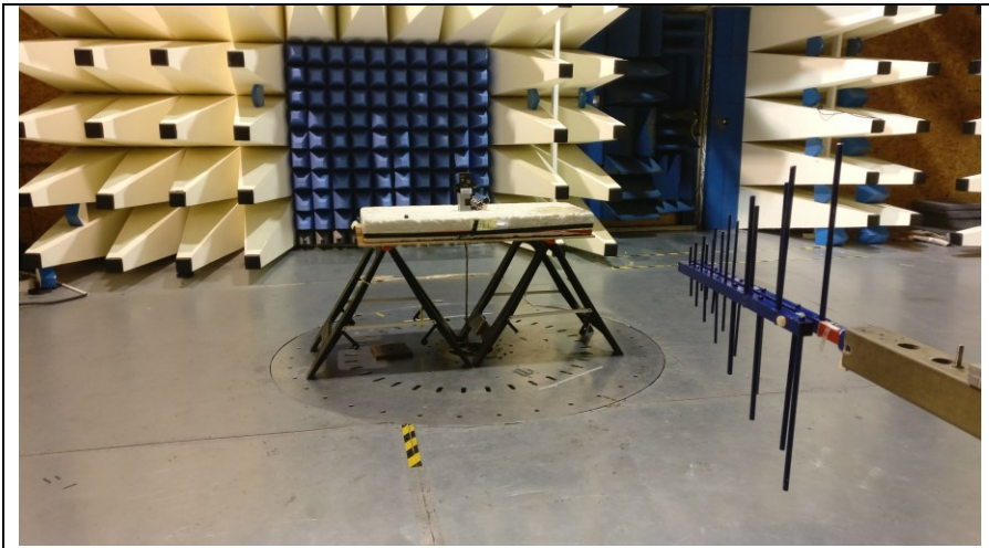
Fig 2a Test setup 300MHz -1GHz Rad Emissions
