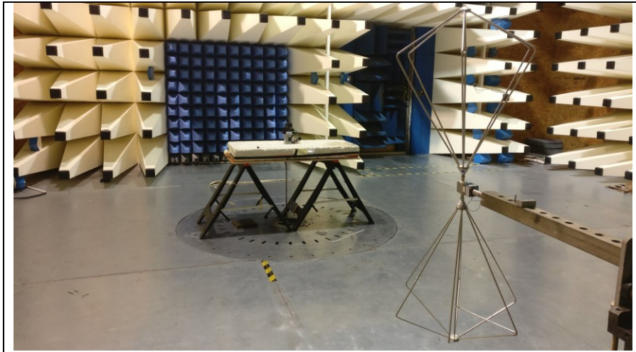
Fig 1a Test setup 30MHz -300MHz Rad Emissions
