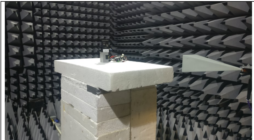
Fig 4 Test setup 18GHz -26GHz Rad Emission 1metre
