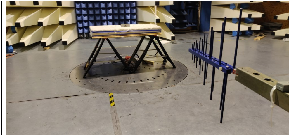
Fig 2a Test setup 300MHz -1GHz Rad Emissions
