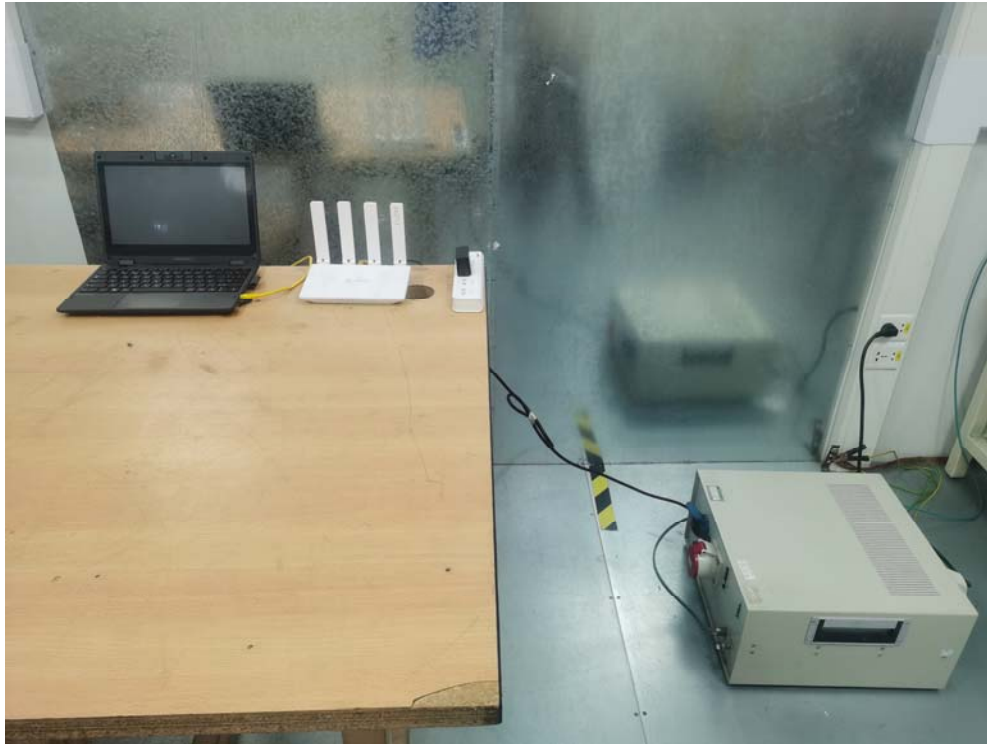
Conducted Emission Test Setup:
