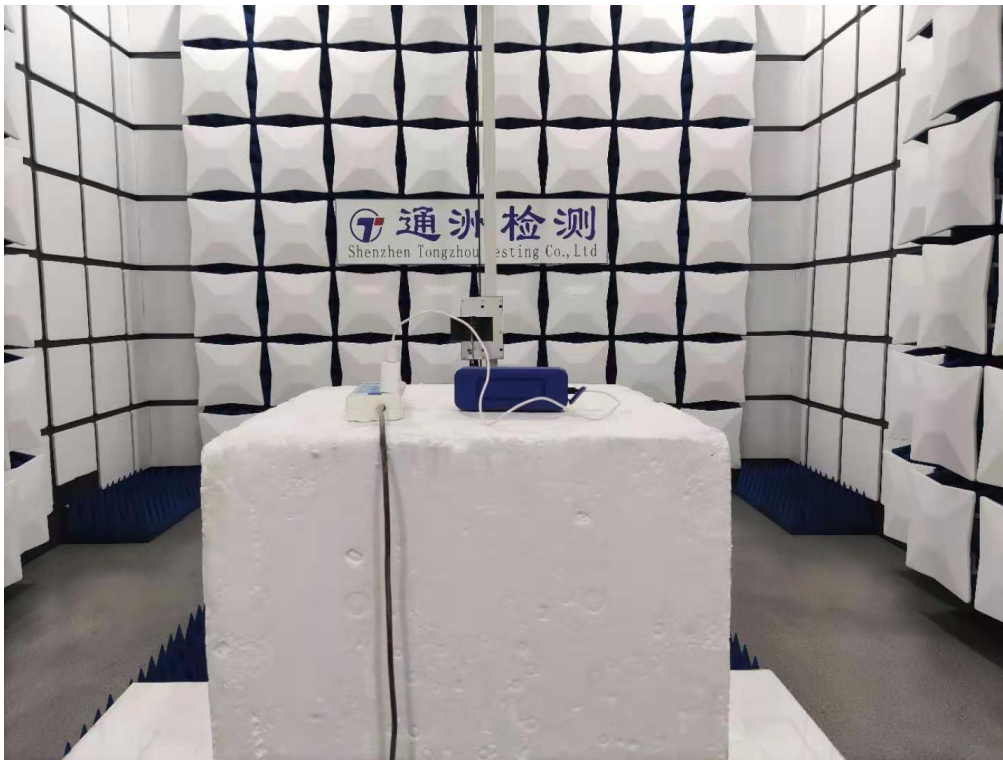
Radiated Emission Above 1GHz
