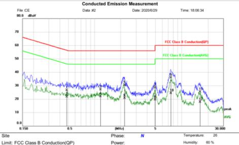
Limit: FCC Class B Conduction(QP) EUT: Haylou Wireless Earbuds
