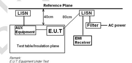
LISN: Line impedence Stabilization Network Test table height=0.8m
