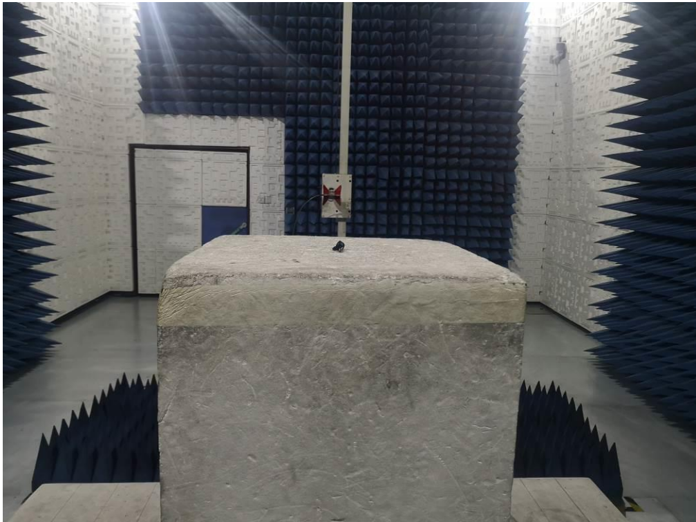
RADIATED EMISSION TEST SETUP ABOVE 1GHz
