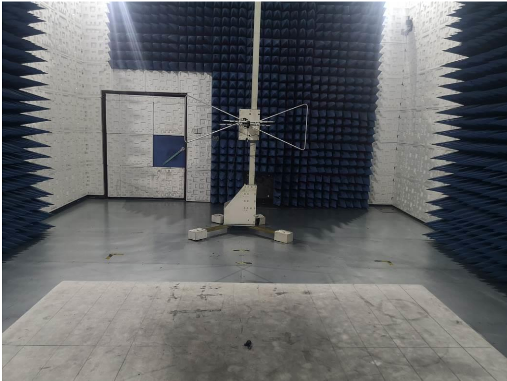
RADIATED EMISSION TEST SETUP ABOVE 1GHz
