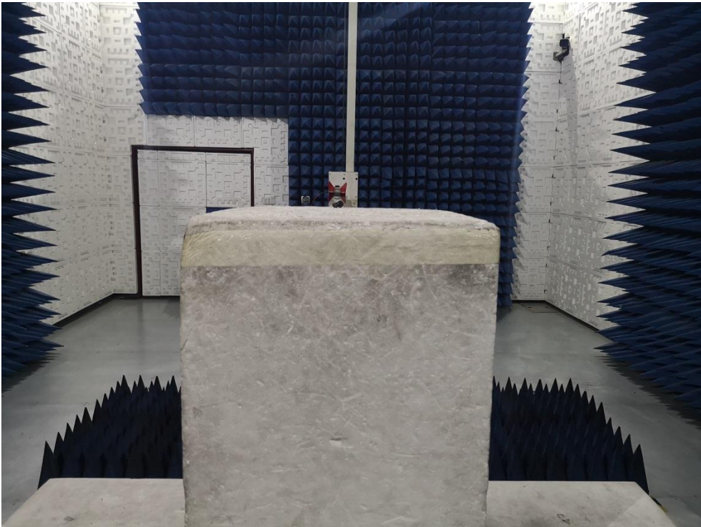
RADIATED EMISSION TEST SETUP ABOVE 1GHz
