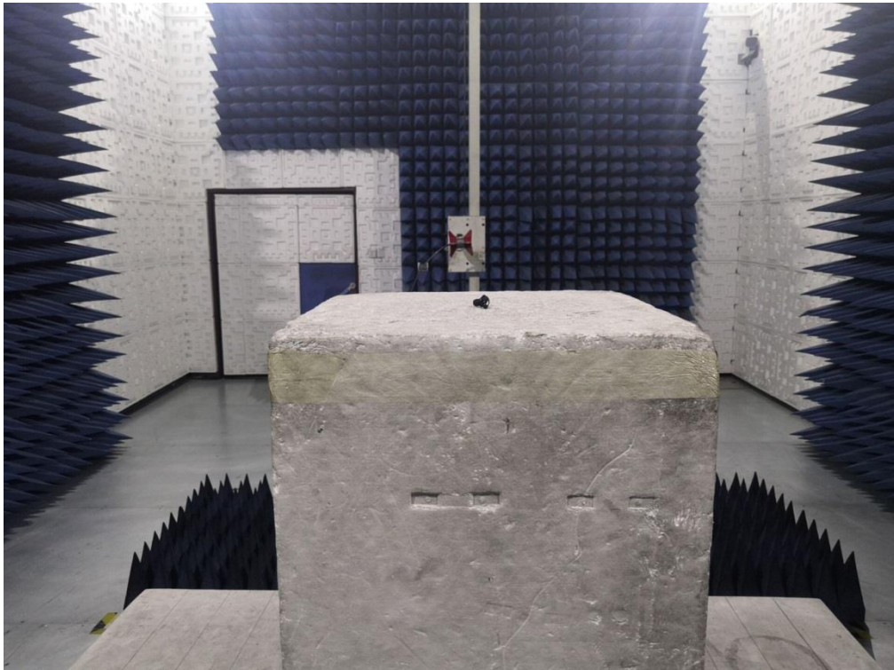
RADIATED EMISSION TEST SETUP ABOVE 1GHz
