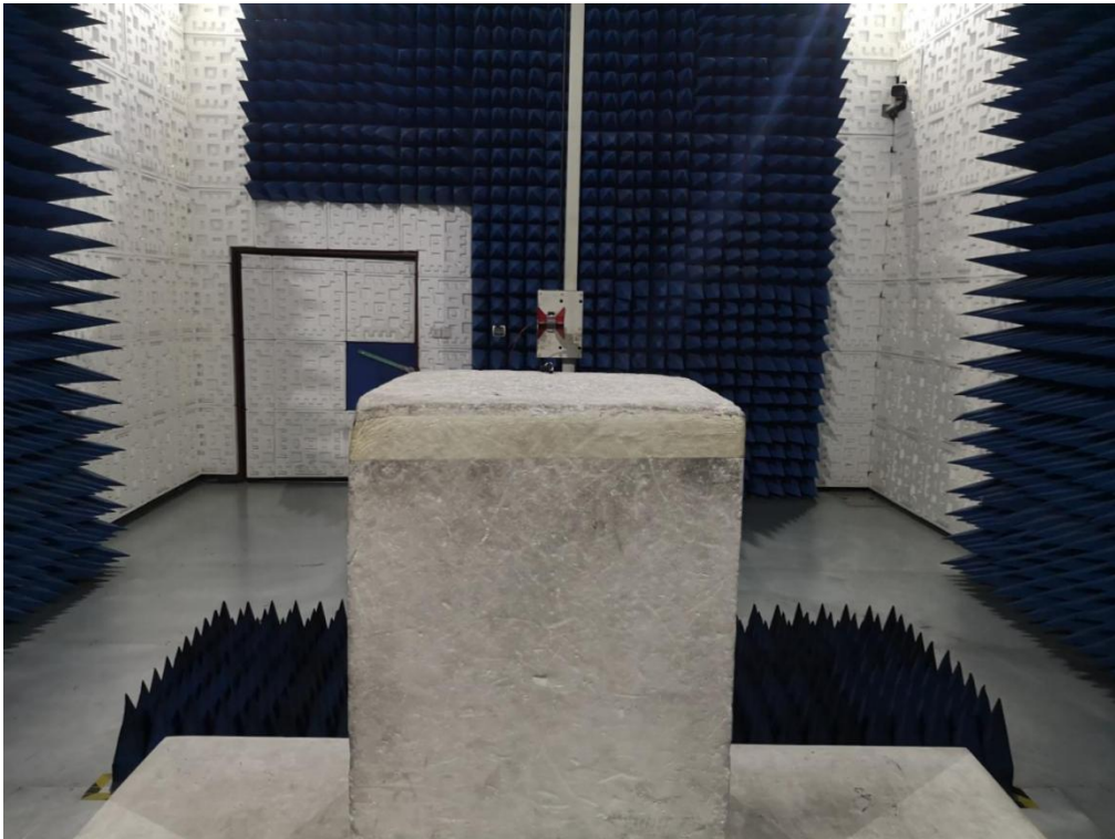
RADIATED EMISSION TEST SETUP ABOVE 1GHZ
