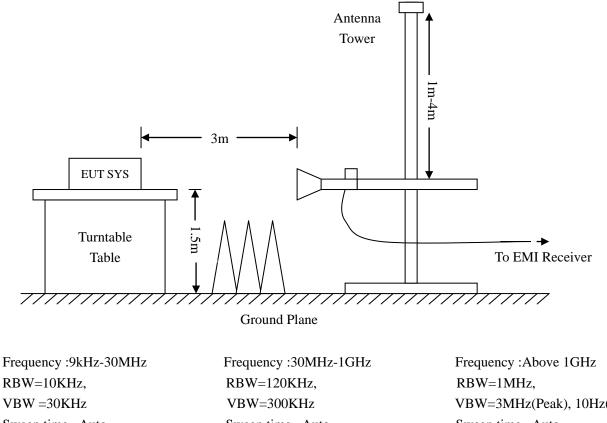
VBW =30KHz Sweep time= Auto Trace = max hold Detector function = peak RBW=120KHz, VBW=300KHz Sweep time= Auto Trace = max hold Detector function = peak, QP RBW=1MHz, VBW=3MHz(Peak), 10Hz(AV) Sweep time= Auto Trace = max hold Detector function = peak, AV
