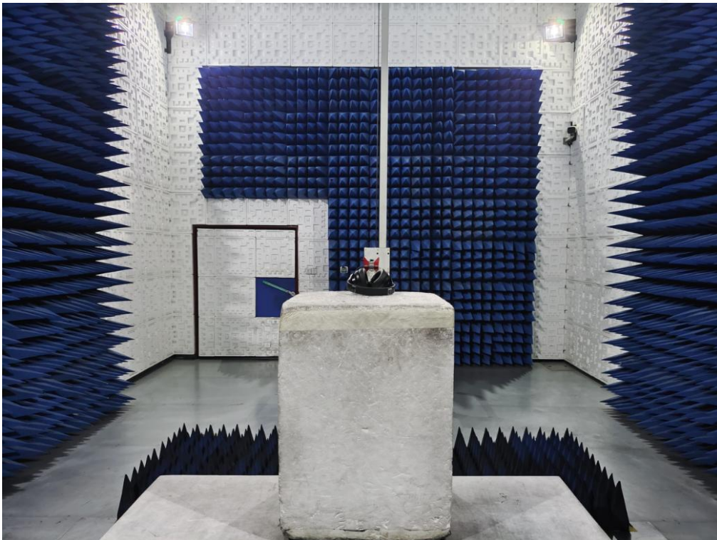
RADIATED EMISSION TEST SETUP ABOVE 1GHZ
