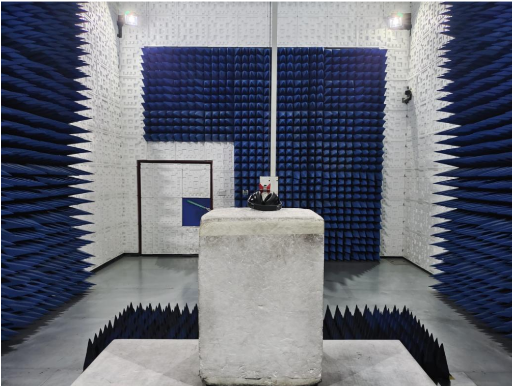
RADIATED EMISSION TEST SETUP ABOVE 1GHz
