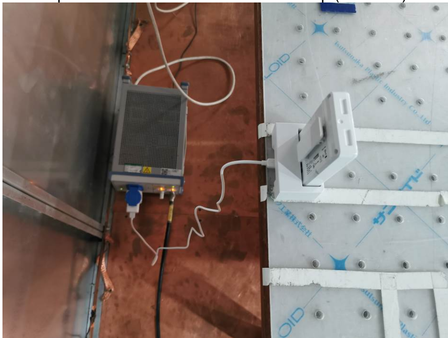
Conducted Emissions Test Setup (with charger)
