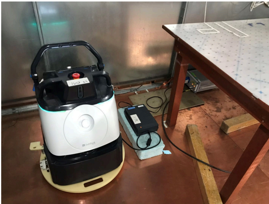
Conducted Emissions Test Setup (with charger)
