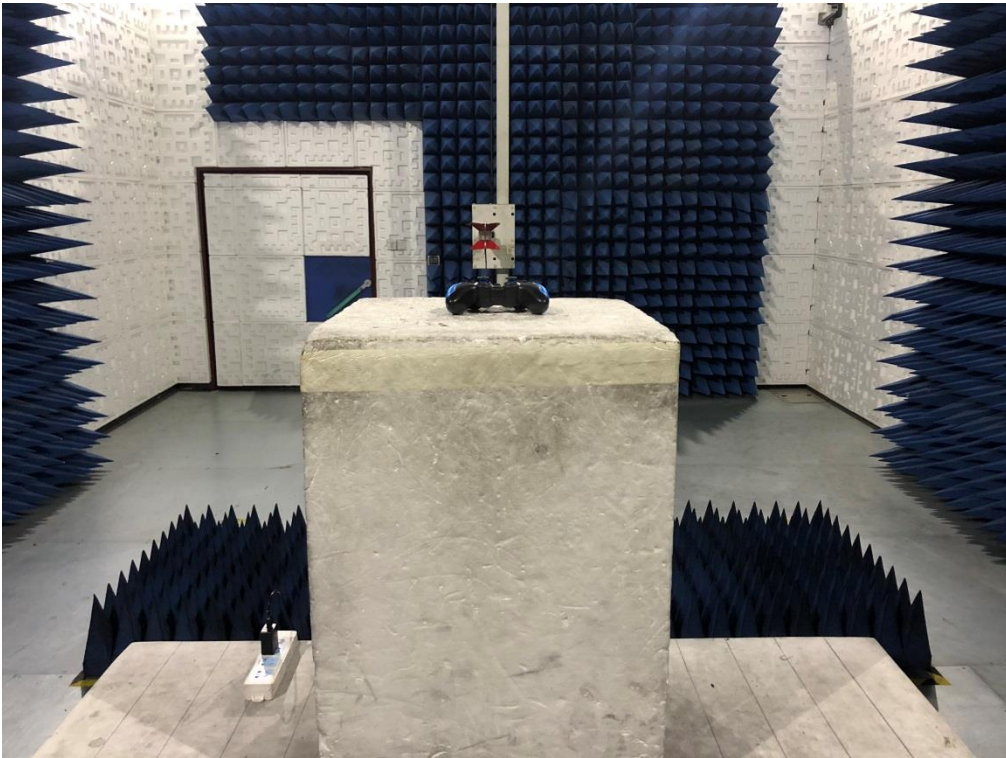
RADIATED EMISSION TEST SETUP ABOVE 1GHz
