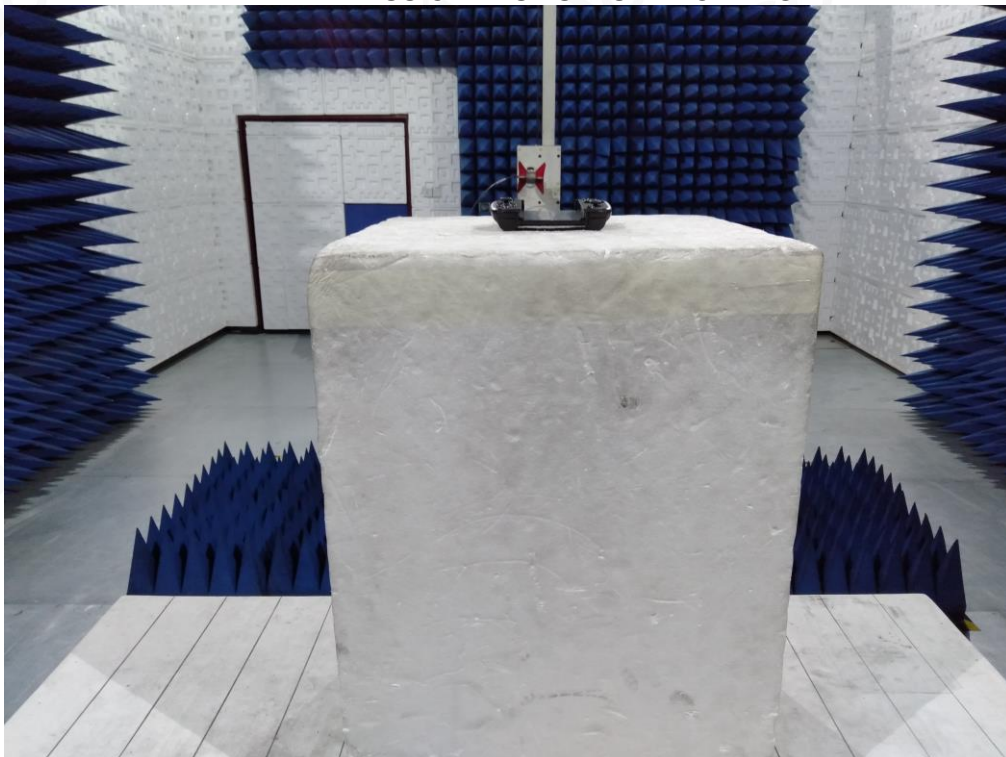
RADIATED EMISSION TEST SETUP ABOVE 1GHZ
