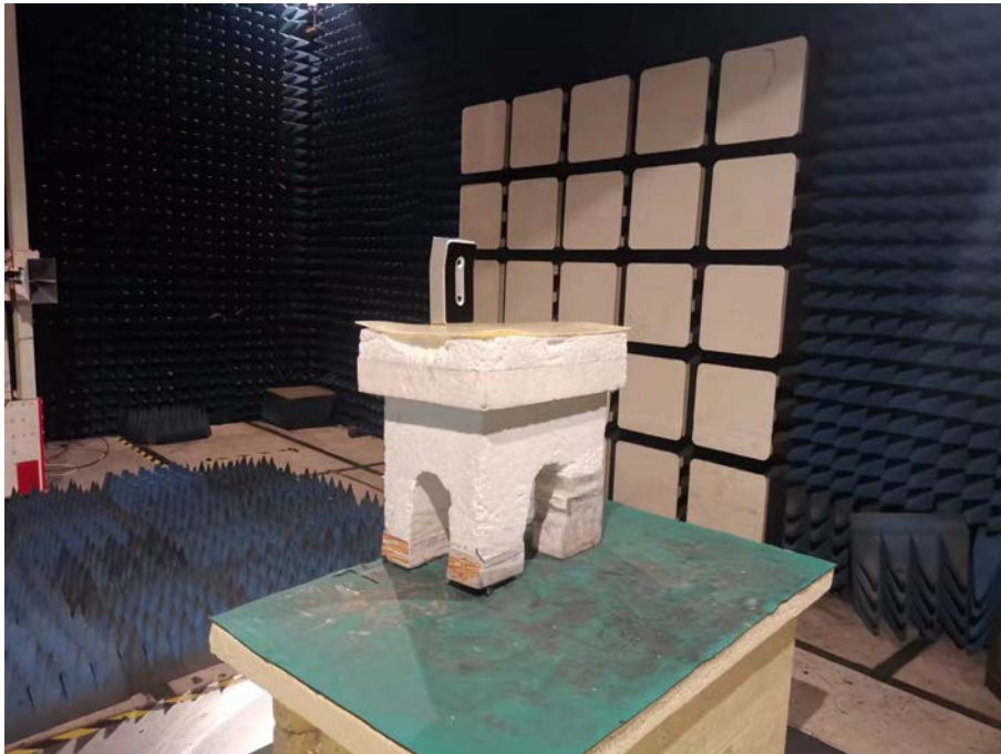
Spurious Emission Test Setup (Above 1GHz)
