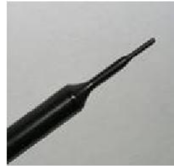
Figure 4.4 EX3DV4 E-field Probe
