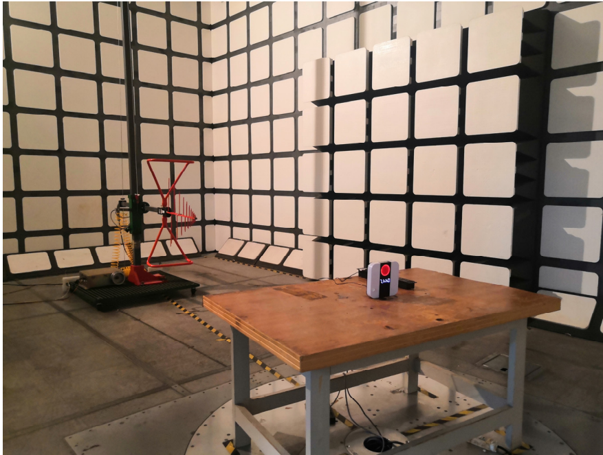
Radiated Emissions View (Below 1 GHz)
