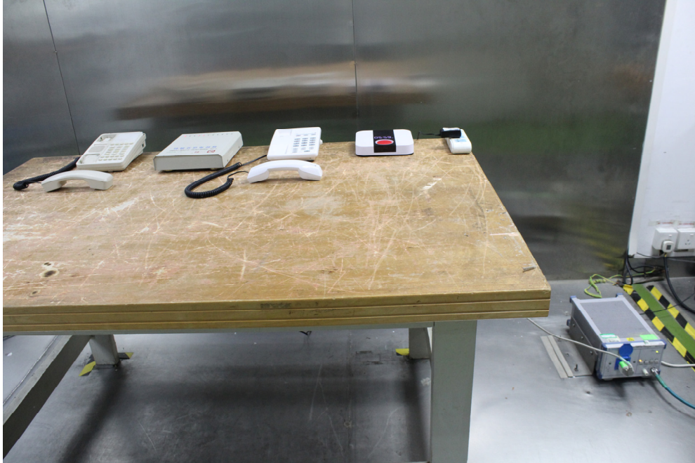
Conducted Emissions - Front View
