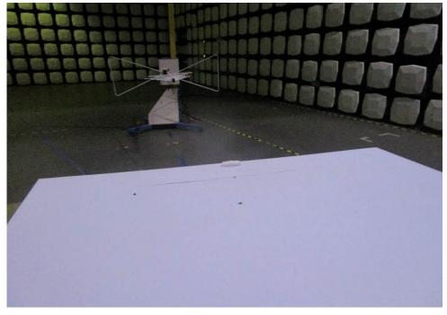
Field Strength of the Fundamental Signal (15.231(b))
