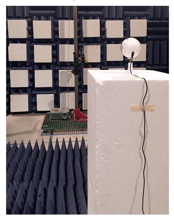
4. Test for Radiated Emissions with SAS-540, 30-300MHz
