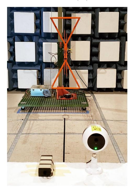
7. Test for Radiated Emissions with SAS-571, 1-7GHz
