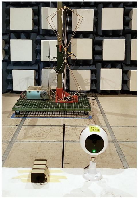
5. Test for Radiated Emissions with VUSLP9111B, 300-1,000MHz
