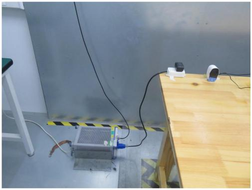
Description: Back View Conducted Emission Test Setup for Power Port
