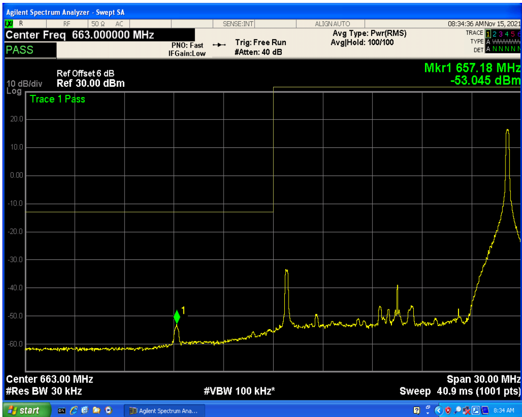
Band71 QPSK BW=15MHz Channel=133197 RB Size=1 Position=#0
