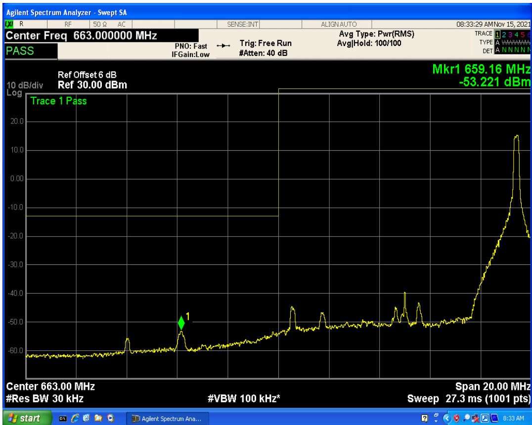
Band71 QAM16 BW=10MHz Channel=133172 RB Size=50 Position=#0
