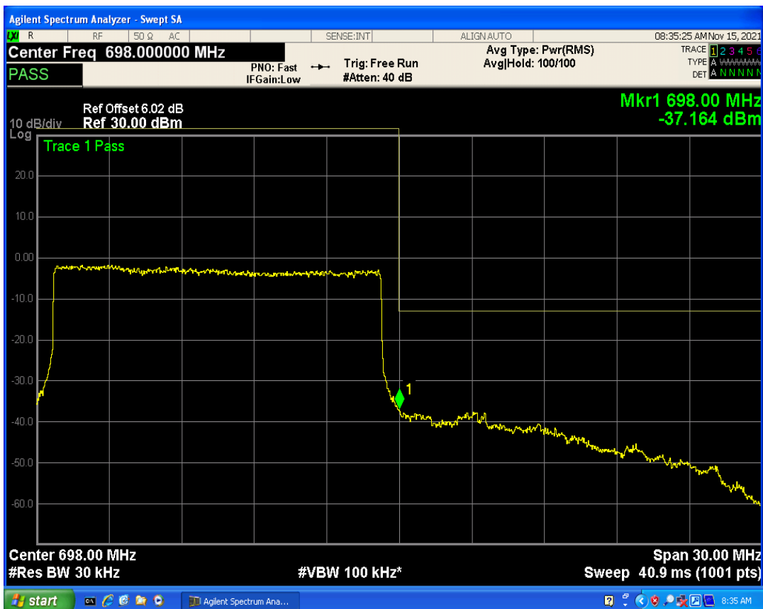
Band71 QAM16 BW=15MHz Channel=133397 RB Size=1 Position=#Max
