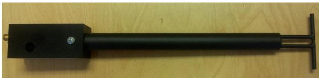
Figure 1 – MVG COMOSAR Validation Dipole
