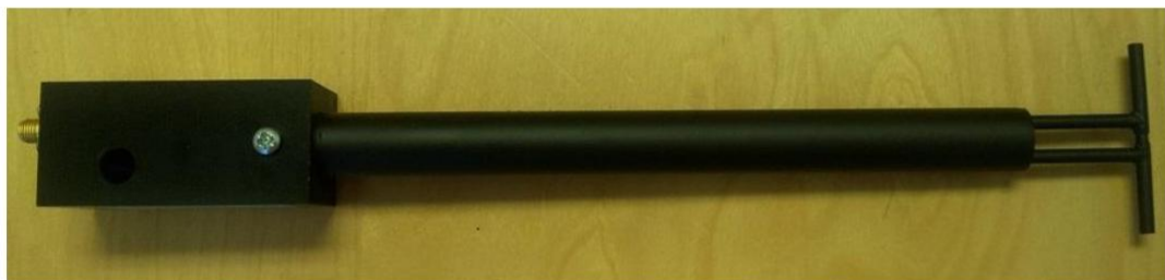
Figure 1 – MVG COMOSAR Validation Dipole
