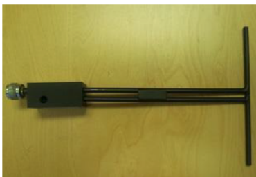
Figure 1 – MVG COMOSAR Validation Dipole
