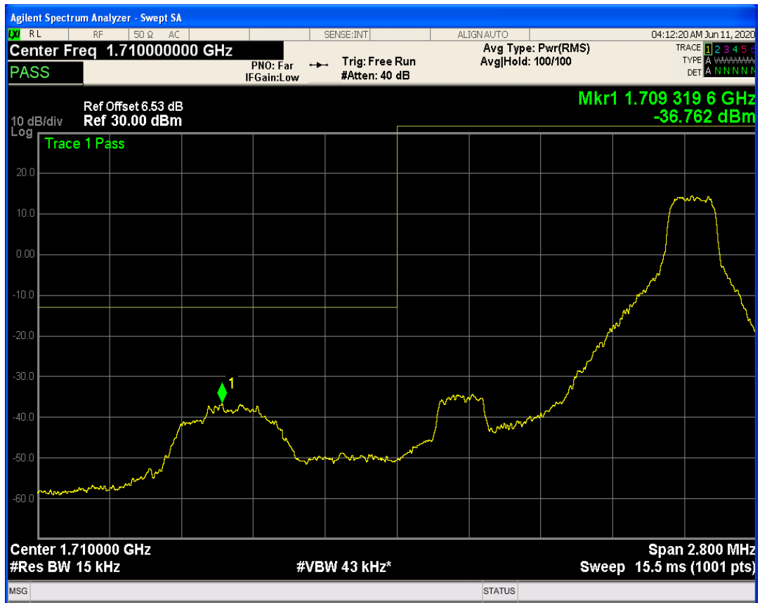
LTE Band66 QAM16 BW=1.4MHz Channel=131979 RB Size=1 Position=#0
