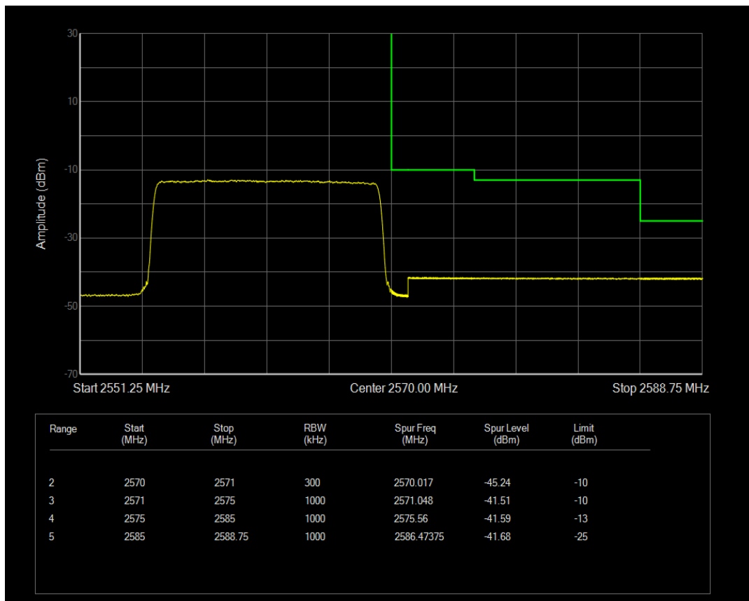
LTE Band7 QPSK BW=20MHz Channel=20850 RB Size=1 Position=#Max
