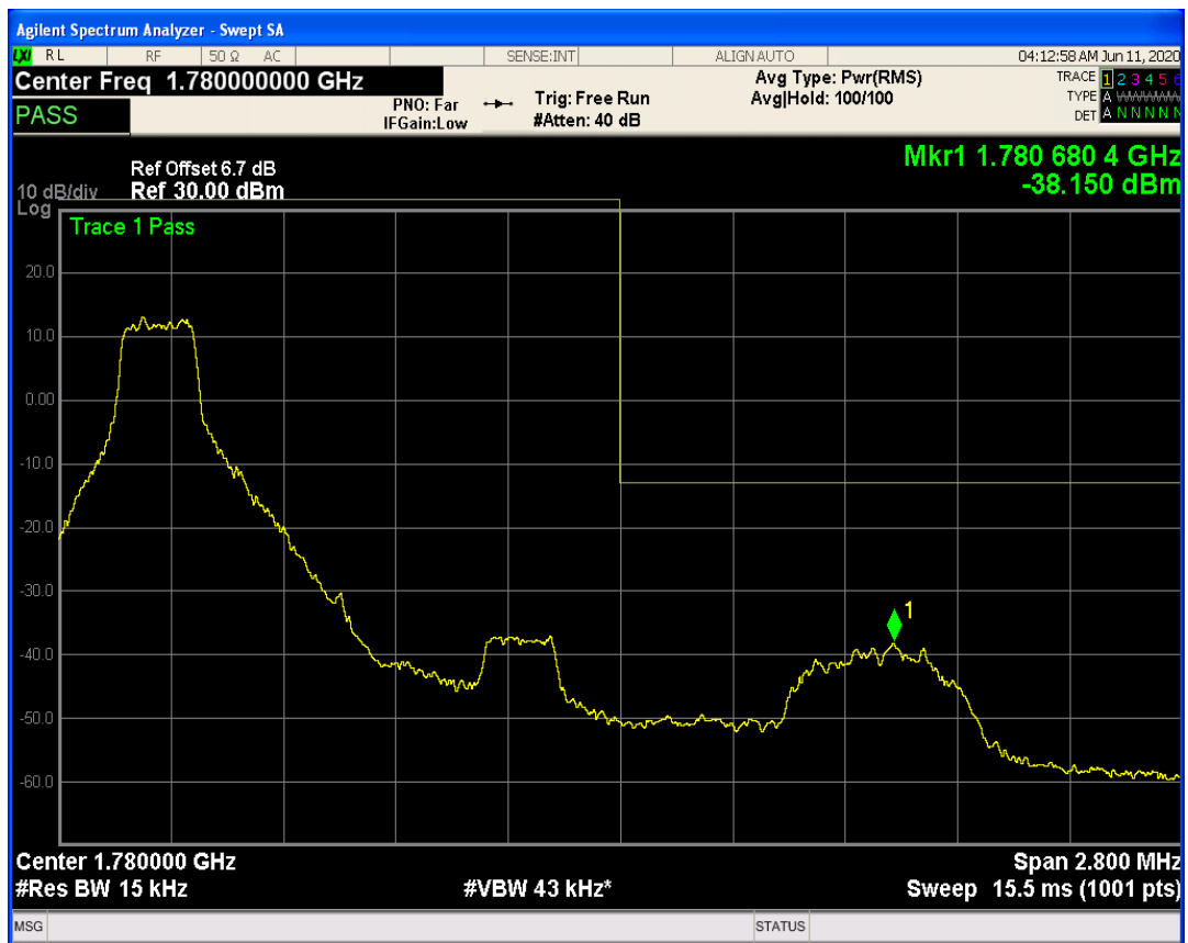
LTE Band66 QAM16 BW=1.4MHz Channel=132665 RB Size=1 Position=#Max
