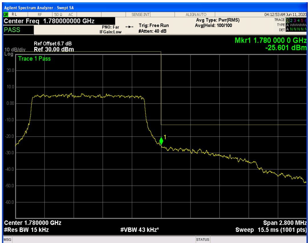
LTE Band66 QAM16 BW=1.4MHz Channel=132665 RB Size=1 Position=#0
