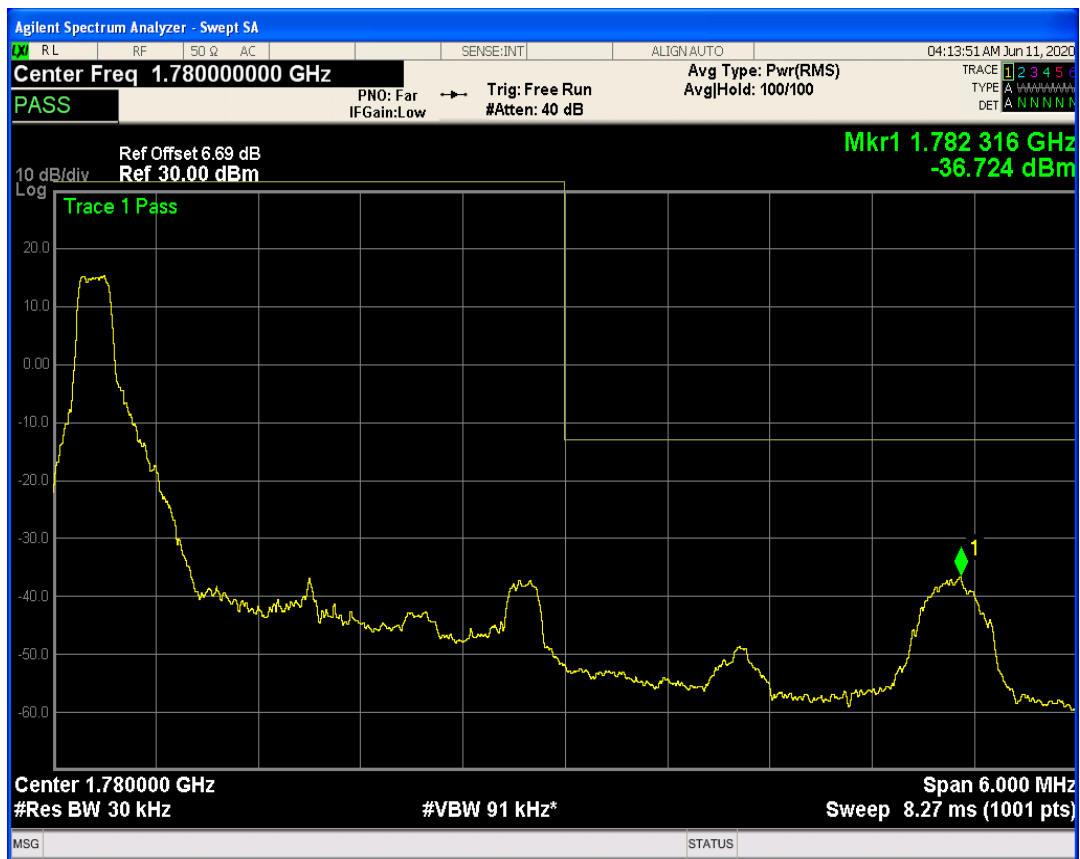
LTE Band66 QAM16 BW=3MHz Channel=132657 RB Size=1 Position=#Max
