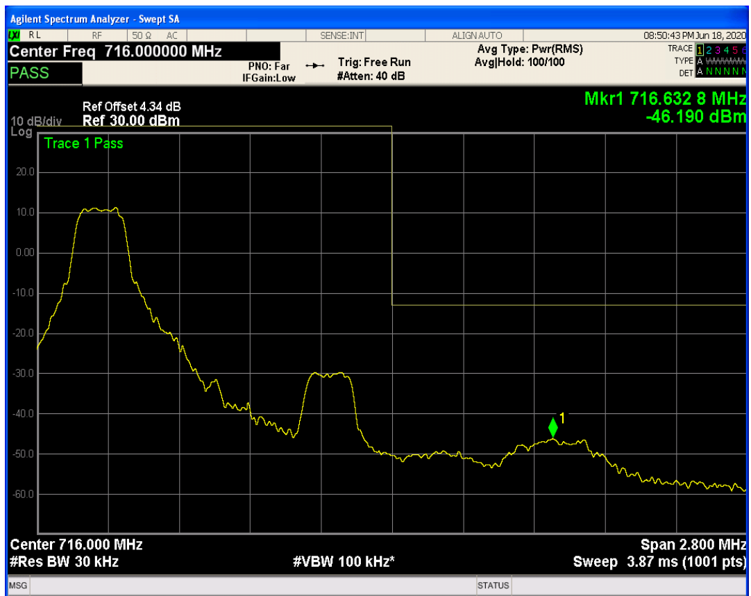
LTE Band12 QPSK BW=1.4MHz Channel=23173 RB Size=1 Position=#Max
