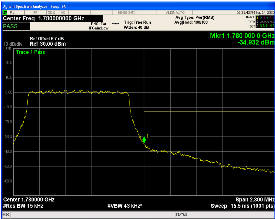
LTE Band66 QAM16 BW=1.4MHz Channel=132665 RB Size=1 Position=#Max
