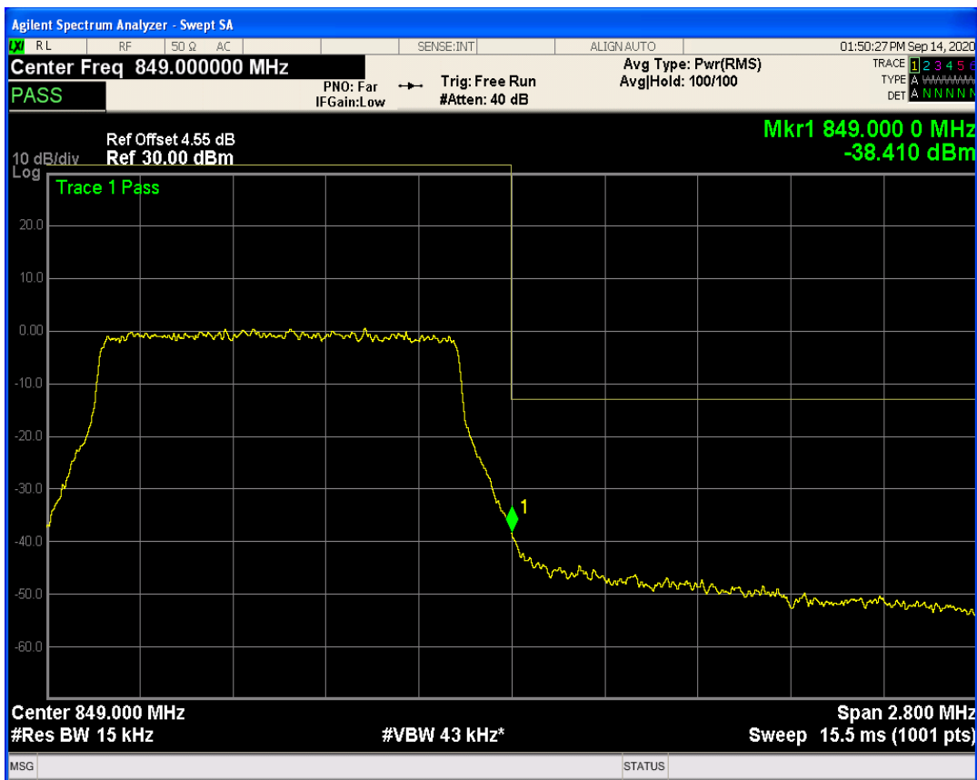
LTE Band5 QAM16 BW=3MHz Channel=20415 RB Size=1 Position=#0
