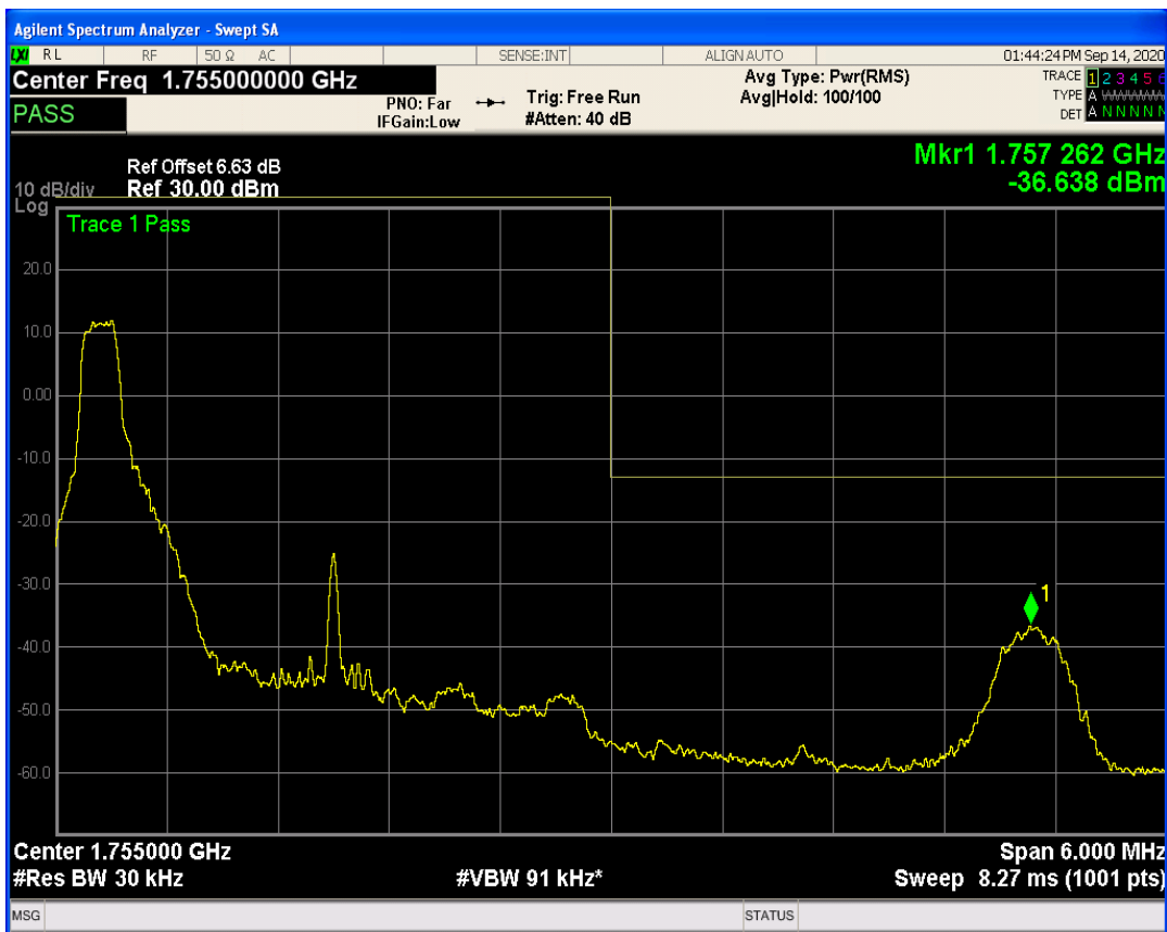
LTE Band4 QPSK BW=3MHz Channel=20385 RB Size=1 Position=#Max
