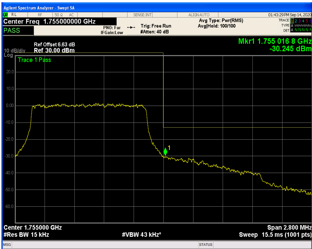
LTE Band4 QPSK BW=3MHz Channel=19965 RB Size=1 Position=#Max
