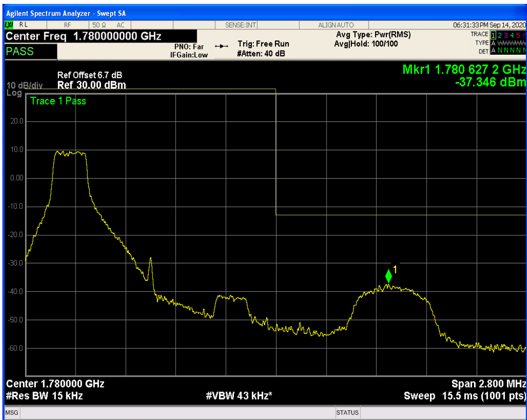
LTE Band66 QAM16 BW=1.4MHz Channel=132665 RB Size=6 Position=#0
