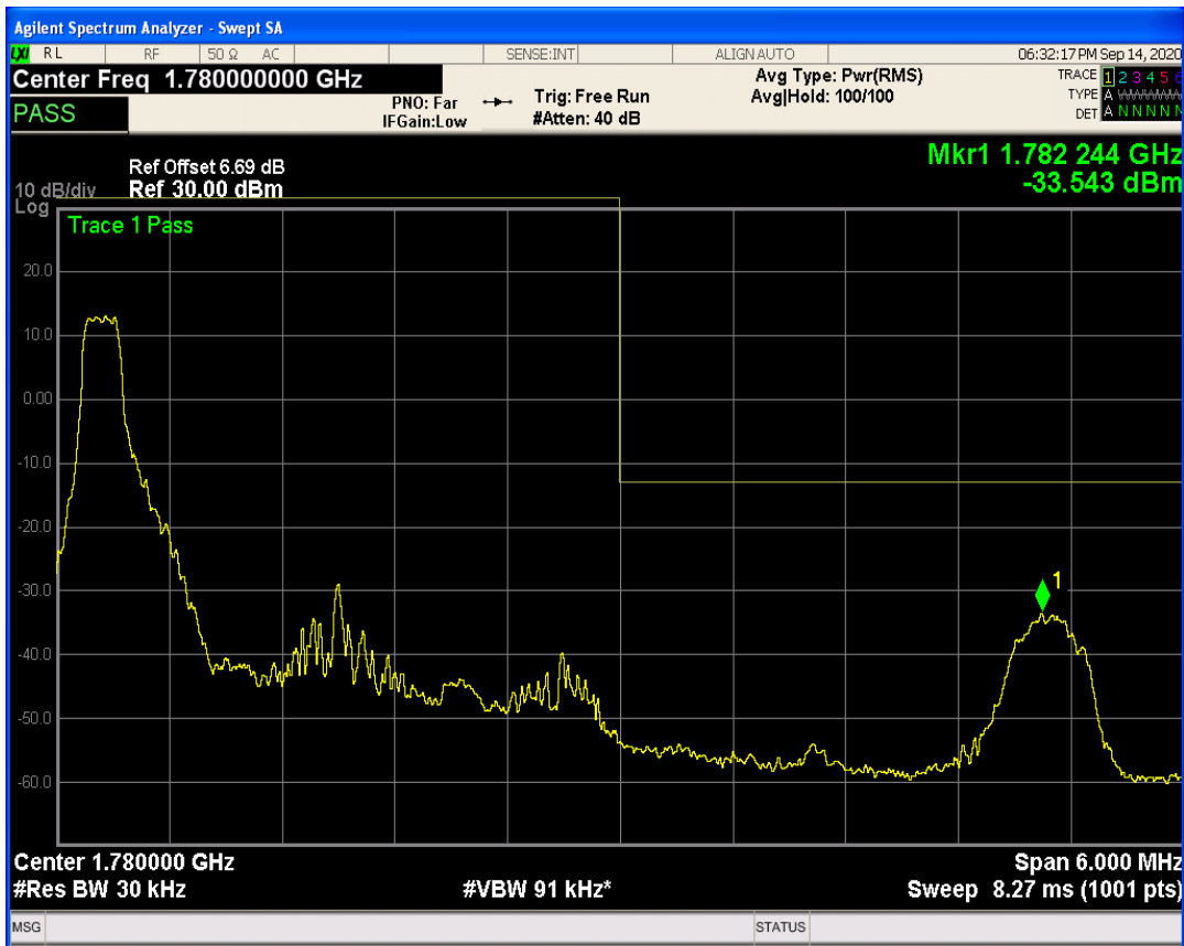
LTE Band66 QPSK BW=3MHz Channel=132657 RB Size=1 Position=#Max
