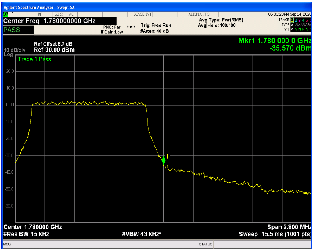
LTE Band66 QAM16 BW=1.4MHz Channel=132665 RB Size=1 Position=#0
