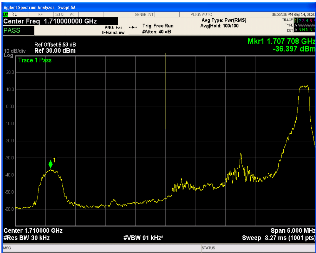
LTE Band66 QAM16 BW=3MHz Channel=131987 RB Size=15 Position=#0
