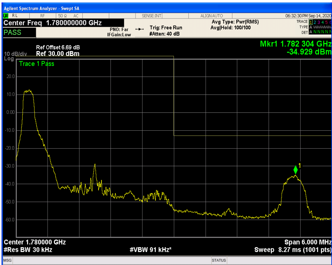
LTE Band66 QAM16 BW=3MHz Channel=132657 RB Size=15 Position=#0
