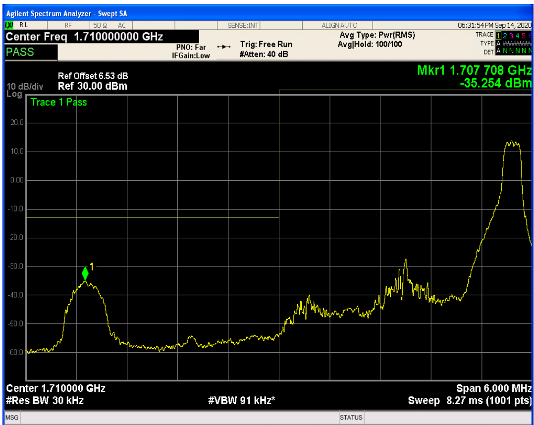
LTE Band66 QAM16 BW=3MHz Channel=131987 RB Size=1 Position=#0
