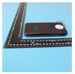
① Wireless charging area for mobile phone which include one coil.
