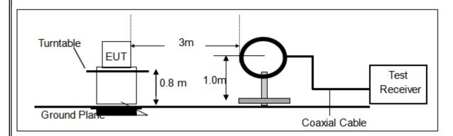
b) For Radiated Emission 30~1000MHz
