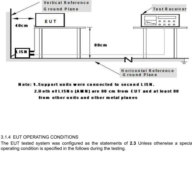
The EUT tested system was configured as the statements of 2.3 Unless otherwise a special
