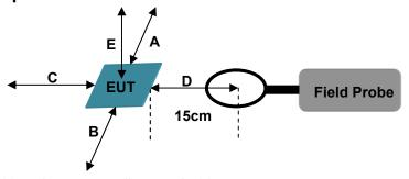
Remrak: The E300 probe antenna diameter is 11.5cm.
