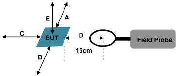
Remrak: The ELT-400 probe antenna diameter is 11cm.
