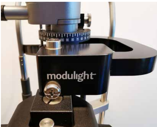
Figure 5. Mounting the ML-SLA to the slit lamp tonometer base.
