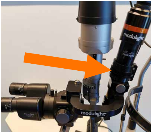
Figure 34. The spot size is selected by rotating the grip wheel on the SLA.
