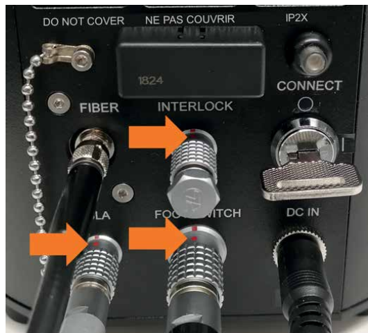
Figure 9. Attach the SLA, interlock and foot switch connectors red dot upwards.
