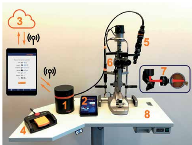
Figure 4. Example setup of ML6710i on an ophthalmic treatment station.
