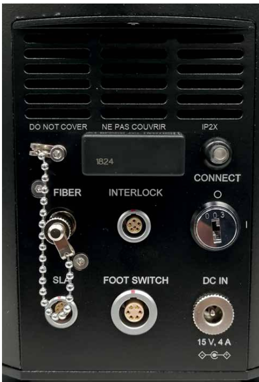
Figure 8. ML6710i rear panel and connections.
