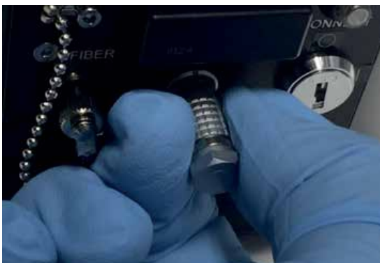
Figure 10. Hold the connector by the grid-surfaced barrel only.
