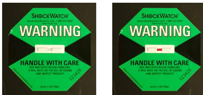
Figure 2. Intact and activated shock indicator. The red indicator on the right side indicates that the ML6710i has been exposed to a potentially damaging impact during transit.
