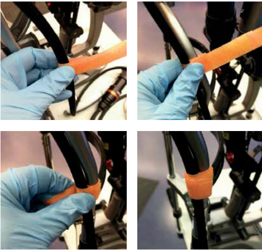
Figure 6. Securing the ML-SLA fiber to the slit lamp headrest using velcros.
