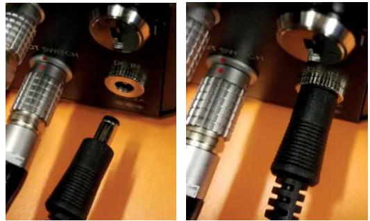
Figure 12. Connecting the power supply cable to the DC IN jack on the ML6710i rear panel.
