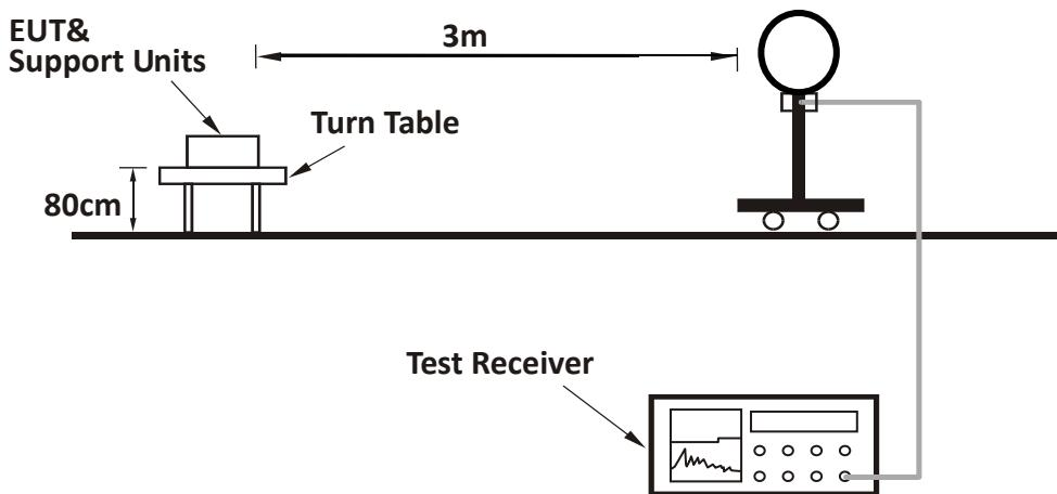
For Radiated emission 30MHz to 1GHz:
