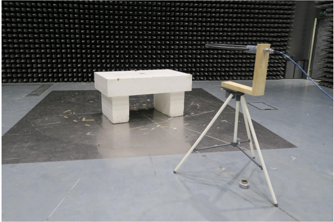
c. High angle front view of EUT on setup table, antenna axis Z
