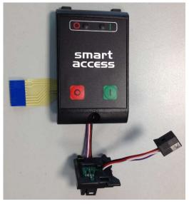
The reader supports the two main frequencies for RFID cards. At the low frequency 125 kHz, a wide range of available transponders are read. At the high frequency 13.56 MHz, the standards ISO14443a and ISO15693 are implemented. NFC devices are detected. The readable card range can be extended.
