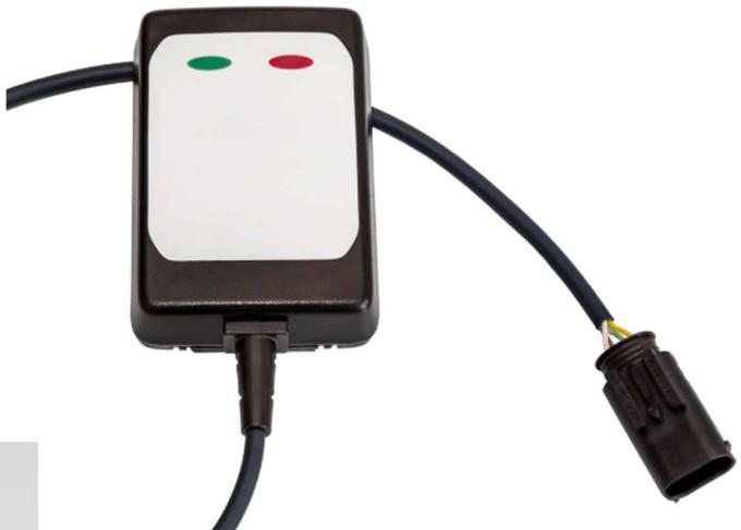
The reader supports the two main frequencies for RFID cards. At the low frequency 125 kHz, a wide range of available transponders are read. At the high frequency 13.56 MHz, the standards ISO14443a and ISO15693 are implemented. NFC devices are detected. The readable card range can be extended. The reader implements the physical interface to the CAN bus. Two LED's indicate the acceptance or rejection of the card.
