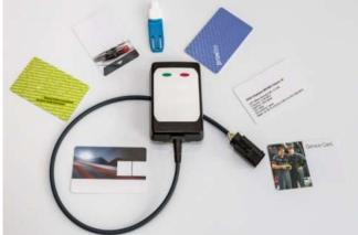
The reader supports the two main frequencies for RFID cards. At the low frequency 125 kHz, a wide range of available transponders are read. At the high frequency 13.56 MHz, the standards ISO14443a and ISO15693 are implemented. NFC devices are detected. The readable card range can be extended.
