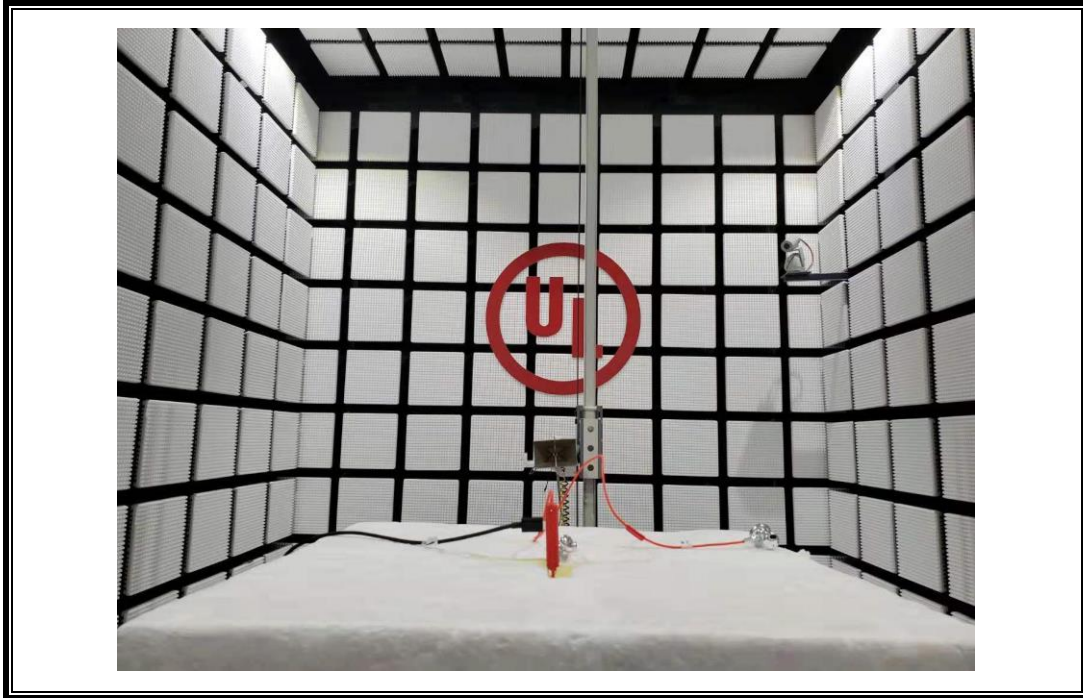
POWERLINE CONDUCTED EMISSIONS MEASUREMENT SETUP
