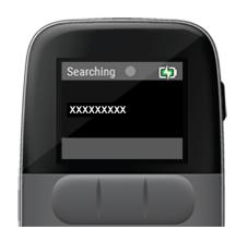
The remote will display *Searching* and the last connected pump's serial number until the pump is paired to the remote. See "Pair to a Spare Pump" on page 118.
