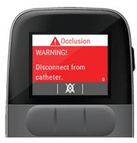
An occlusion occurs when the tubing or catheter is blocked or partially blocked from delivering your medication.
