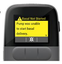
makes the attention alarm sound and the remote interface will display a Basal Not Started Attention Alarm.
