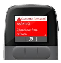
When the pump detects that the cassette is removed without being commanded to stop delivery, a Cassette Removed Alarm displays.
