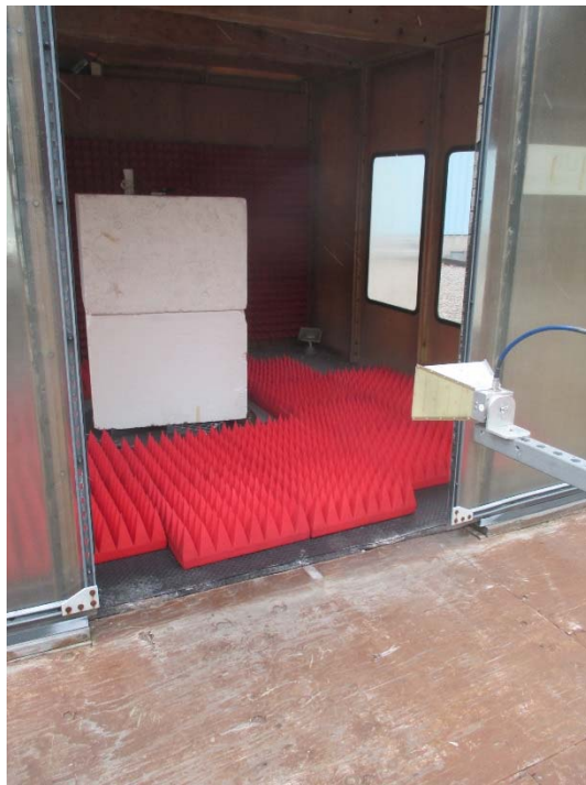
Vertical Antenna Polarization
