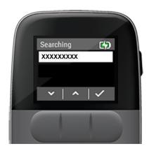
5. On the remote, use to highlight the pump's serial number and press.
