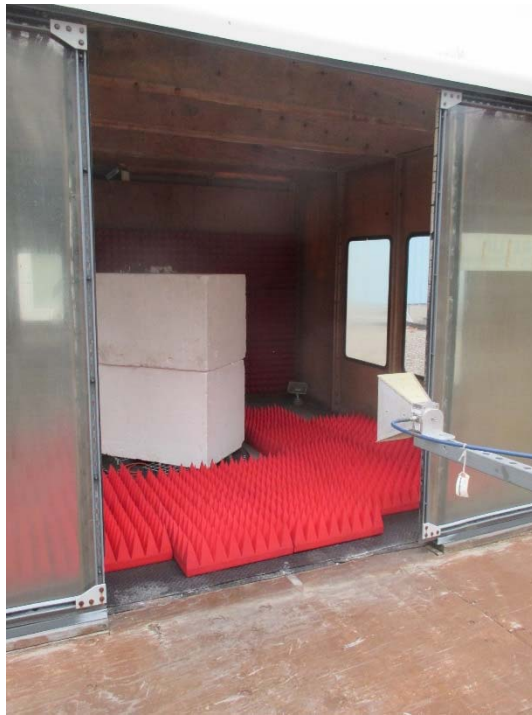
Horizontal Antenna Polarization
