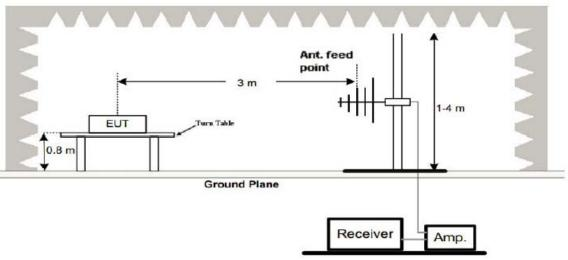
(3) Radiated Emission Test-Up Frequency Above 1GHz
