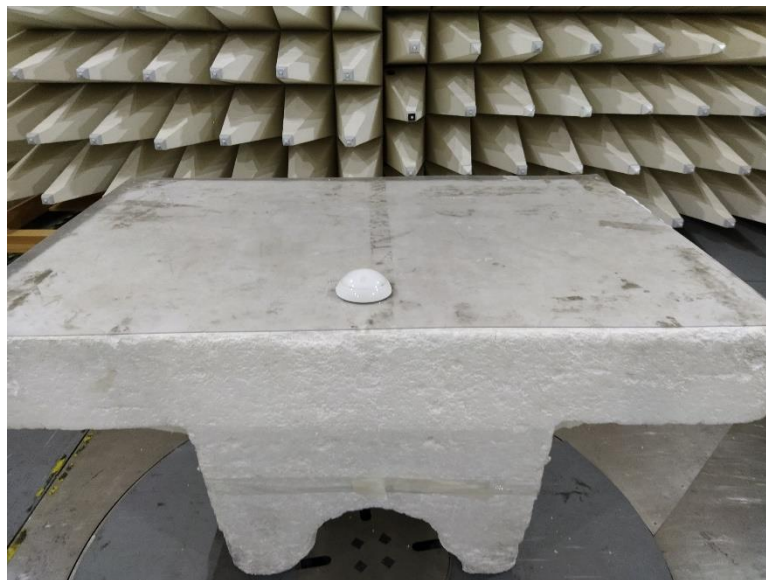
Photograph 8.1.2 Setup for final radiated emission measurements, EUT cabling
