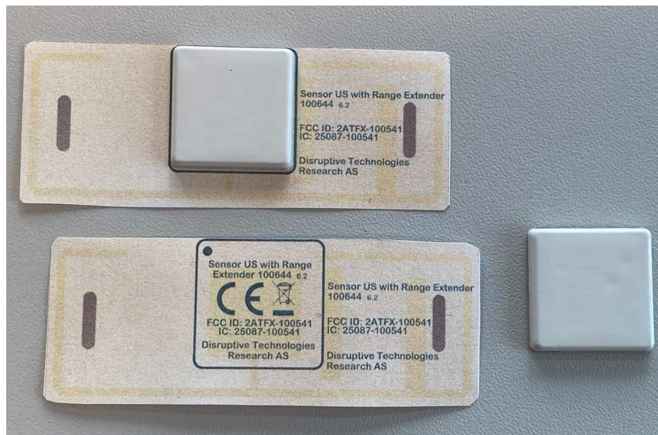
Figure 1: Top: Image of front side of PN 100644 Sensor US with Range Extender, fully assembled by end user. Bottom: PN 100644 Sensor Range Extender PCB (EU & US) (left) and Sensor US with FCC ID: 2ATFX-100541 (right) as shipped to customers, not assembled.
